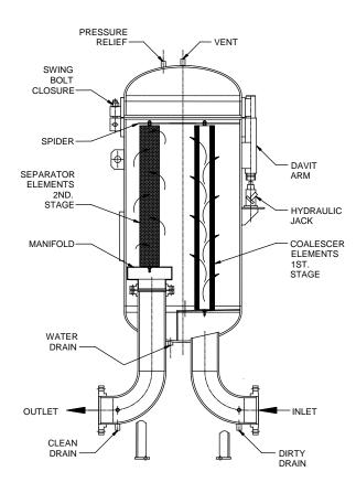
**INFILTEK** filter separators are designed to separate two immiscible liquids and remove particulate contamination through a two stage coalescer - separator process.
