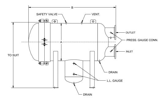
The horizontal filter/separator design provides more convenient access to the cartridges than the vertical design. The end opening hinged cover swings open and the mounting assembly for both stages of cartridges is exposed for service. For refuelers and hydrant carts, saddle type legs and short sump is supplied.
